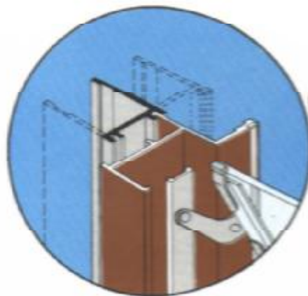
Brick fin allows for installation of window in masonry construction — four positions.
