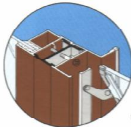
Mullion joins two windows side by side causing outside flanges to touch each other creating a flush interior. Mullion does not add to overall dimension of windows.
